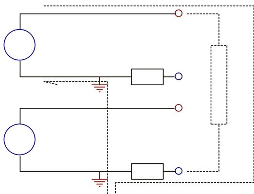
Because one point in the test low end of each unit structure is connected to the ground. Current is collected between the low end of the test and ground. The current loop of the high voltage of adjacent units can be achieved through the low end of the other units. The effect of this current on the measurement is as follows:
