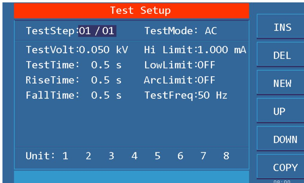
**Figure 4.2.2 AC SETUP Interface**
