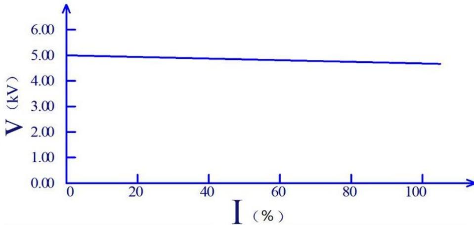
**Figure 3-3 AC voltage load regulation**
