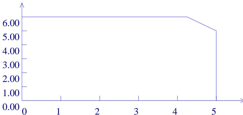
**Figure 3-4 TH9010/A DC Voltage Output Range**
