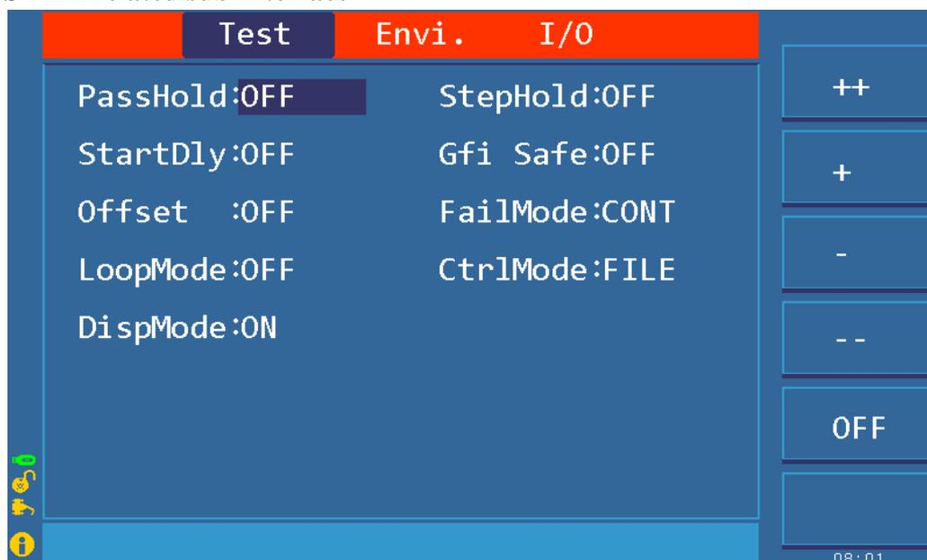
Figure 4.2.3.1 Test SYSTEM related interface
