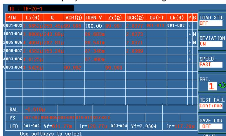
When <TRANS ID> displays Ignore Nom:SKP TEST LIMITED DEV, the deduction can't be succeeded due to the deviation between test value and nominal value is too large; now user has to check the contact if reliable or the standard sample is correct
