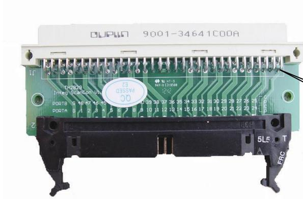
Interface board for 24-channel to 20-channel
