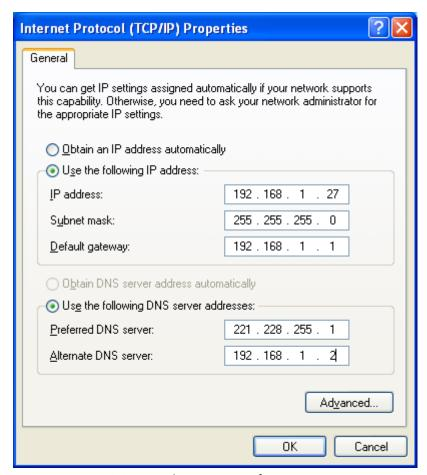
Figure 6-6 Network Parameters of Host computer
