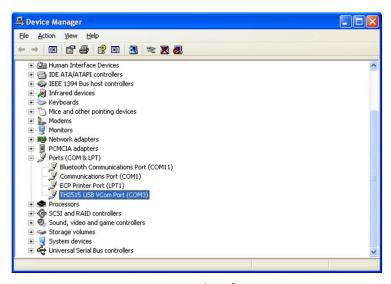
Figure 6-13 VCom Display of PC Device Manager
