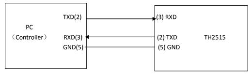
Figure 6-1 Connection of the instrument with PC
