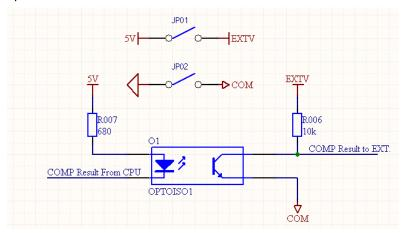
External control signal input circuit is shown as follows:
