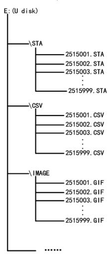
Figure 4-2 file structure in a U disk
