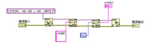
Figure 6-9 Access to TH2515 through Labview
